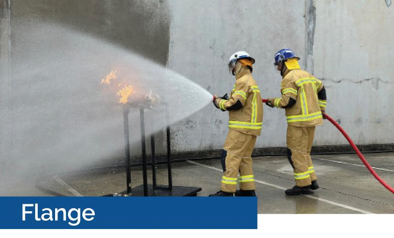
The Gasworks' Flange Live Fire Training Device is designed to simulate a real-life flange fire scenario, producing intense flames and authentic heat.
