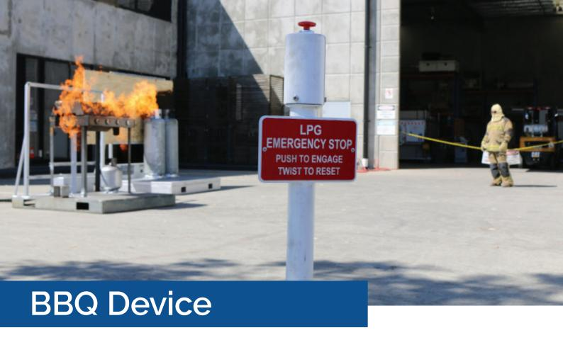
The Gasworks' BBQ Live Fire Training Device is designed to simulate a real-life backyard emergency scenario, producing intense flames and authentic heat.
