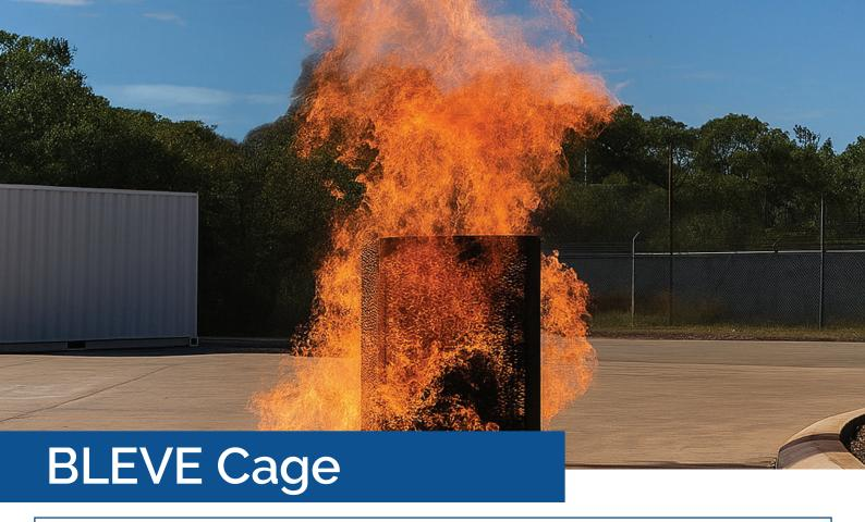
The Gasworks' Boiling Liquid Expanding Vapour Explosion (BLEVE) Cage offers the safe detonation of pressurised vessels, providing an invaluable training tool for emergency responders and industrial personnel.
